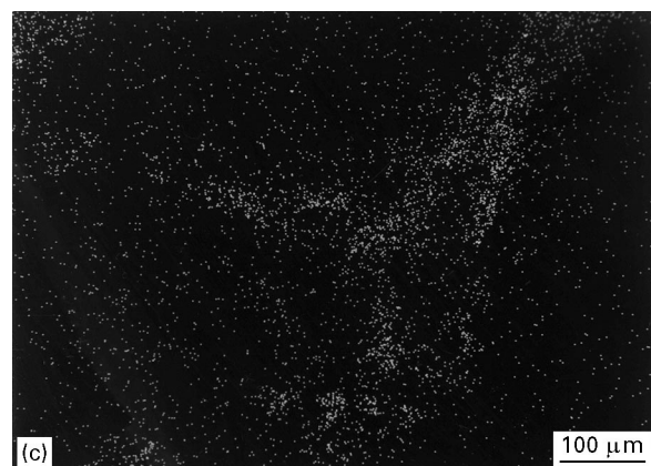
Figure 6 Scanning electron micrograph of the alumina particulates in the as-received condition. (b) Scanning electron micrograph of the nickel-deposited alumina particulates removed from the 700 °C CVD–FBR experiment. (c) Nickel elemental X-ray mapping of the nickel deposited alumina particulates removed from the 700 °C CVD–FBR experiment.
